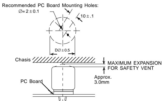
The space from the top of the can shall be more than ⑧(3mm) from chassis or other construction materials so that safety vent has room to expand in case of emergency.
