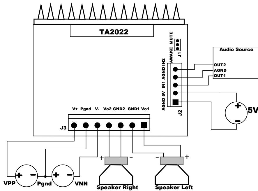
Three external power supplies are required to operate the EB-TA2022: VPP, VNN (referenced to Pgnd), and 5V (referenced to Agnd). The VPP and VNN form a split rail supply referenced to Pgnd. The 5V ground (Agnd) must be kept separate from the VPP and VNN ground (Pgnd). Agnd and Pgnd are joined at a common point on the EB-TA2022 near headers J2 and J3.
